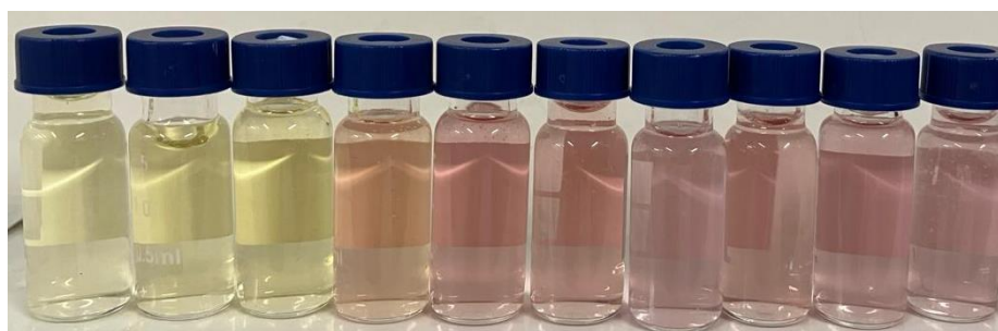
Figure 1. AgNPs dispersions in the presence of different concentrations of CIP, ranging from 0 to 1.7 mg/L.
